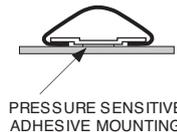
Perhaps the easiest track mounting option is with double sided pressure sensitive transfer tape. Simply apply on a clean, oil-free surface, and allow a 24-hour cure time.
